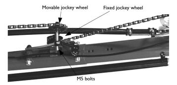
Once the correct position for the rider has been attained, the chain length must be adapted. For each hole pair the jockey wheel has been moved, four links of the chain must be removed.
