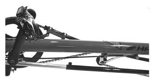
The Steering rod is clamped with a 5 mm Allen bolt. Straighten the front wheel and the handlebar and away you go.
