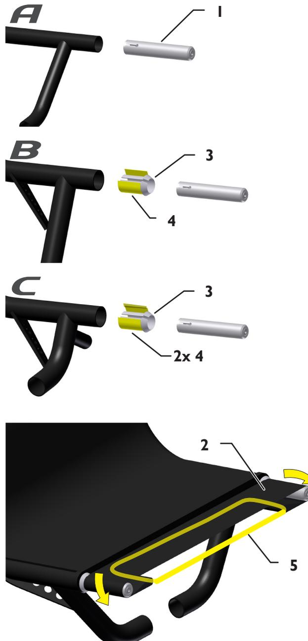
The Seat Extension increases the surface area of the seat or, alternatively, the seat back. This optional feature offers you more space and comfort and is available for the Kettwiesel, Lepus, and Pino.
